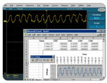
Open Windows Platform. TDS5000 Series waveform display with Excel window and ActiveX toolbar.
