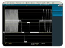
Video Desian. Illustration of triagering on an analog HDTV tri-level sync signal and examining horizontal blanking interval.
